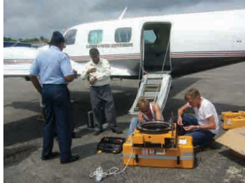
Picture 3-2 Setting up the aerial camera
