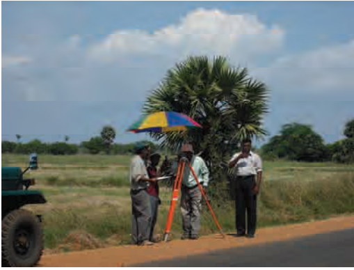
Picture 3-3 Observation of Levelling
