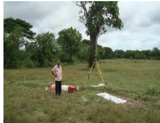
Photo Control Point Survey (GPS Survey)
