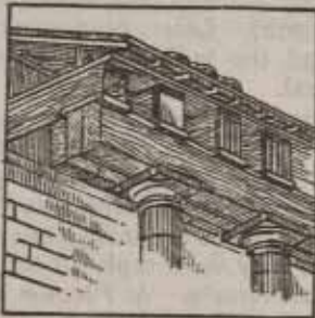
Fig. 376. Wooden prototype of the Doric order.
