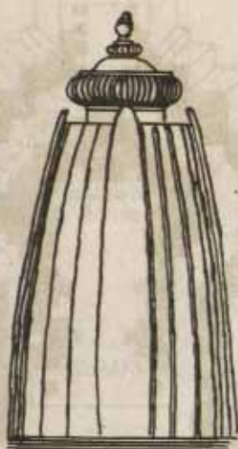
Fig. 168. A Central Indian sikhara, showing the double amalakas and the raha-pagas projecting beyond the gandi.
