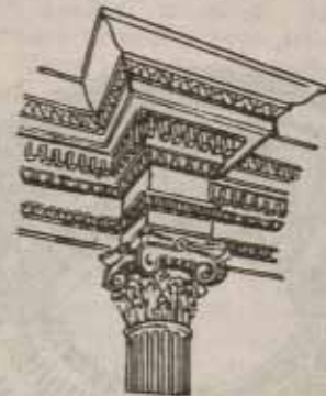
Fig.403. Projecting entablature over capital, triumphal arch, Rome.
