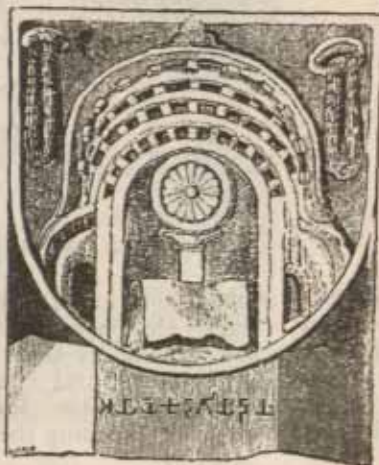
Fig. 46. Front of a chaitya hall, from a bas-relief at Bodhi-Gaya, with imitation of wooden structural details.
