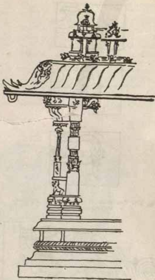
Fig. 210. Mandapam with double-flexed kapota (cornice) and clustered pillar, Vijayanagar period, Hampi.
